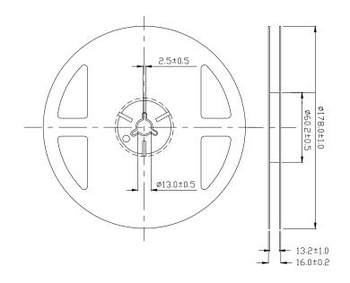
Note: The tolerances unless mentioned are ±0.1, unit=mm. Carrier Taping Dimensions: Loaded Quantity 1000PCS/Reel
