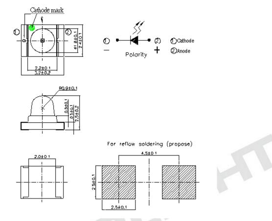
**Notes:** 1.All dimensions are in millimeters 2.Tolerances unless dimensions ±0.1mm
