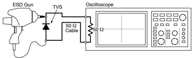
Figure 4. Diagram of ESD Test Setup
