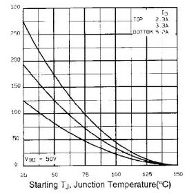
Fig. 12c - Maximum Avalanche Energy vs. Drain Current
