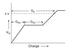
Fig. 13a - Basic Gate Charge Waveform
