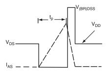
Fig. 12b - Unclamped Inductive Waveforms
