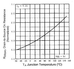
Fig. 4 - Normalized On-Resistance vs. Temperature
