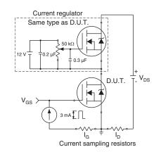
Fig. 13b - Gate Charge Test Circuit
