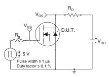
Fig. 10a - Switching Time Test Circuit
