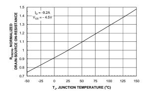
Figure 3. On-Resistance Variation withTemperature.
