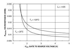
Figure 4. On-Resistance Variation with Gate-to-Source Voltage.
