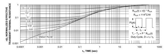
Figure 11. Transient Thermal Response Curve.
