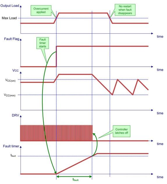
Figure 71. Latched Timer-Based Overcurrent Protection (Options A/E)
