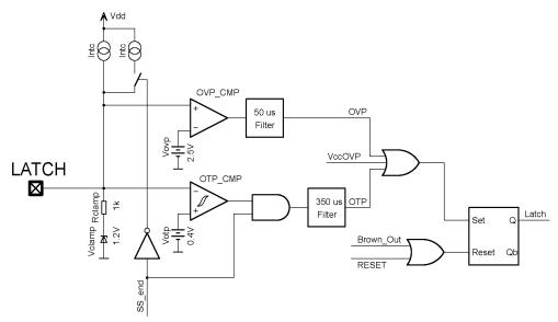
Figure 75. Latch Detection Schematic
