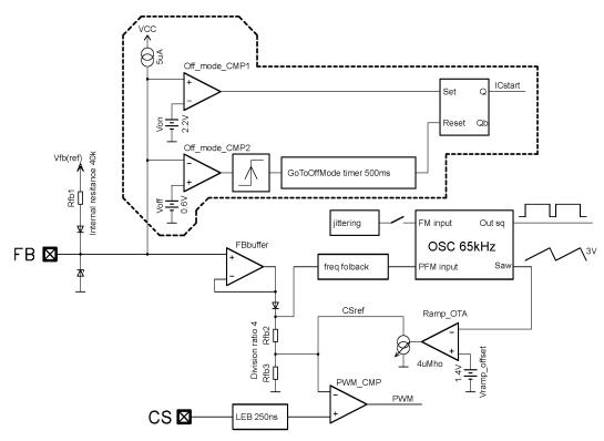
Figure 64. Slope Compensation Block Diagram
