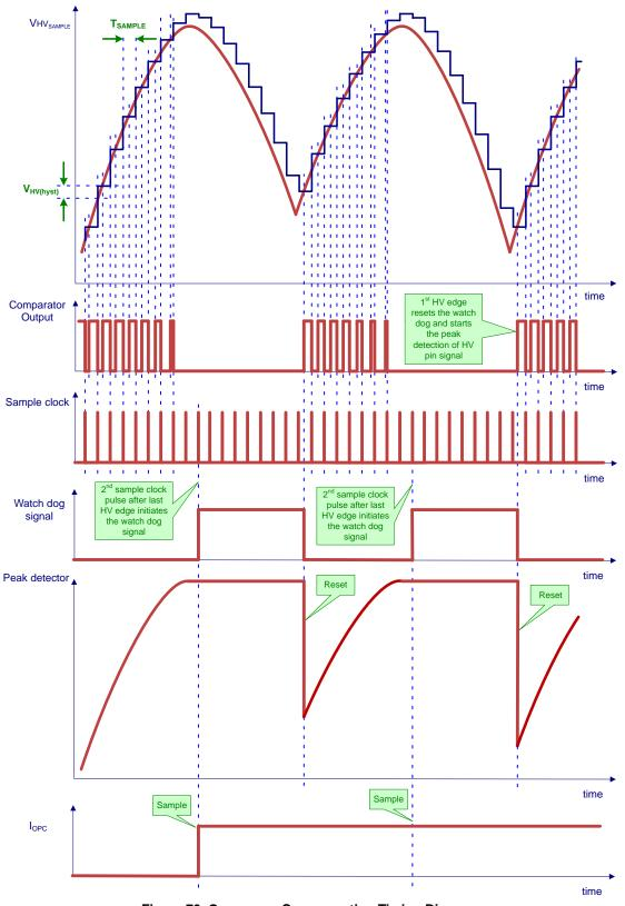
Figure 70. Overpower Compensation Timing Diagram
