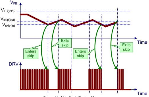
Figure 61. Skip Mode Timing Diagram
