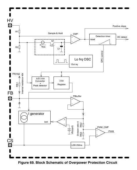
A 3 bit A/D converter with the peak detector senses the ac input, and its output is periodically sampled and reset, in order to follow closely the input voltage variations. The sample and reset events are given by the output from the ac line unplug detector. The sensed HV pin voltage peak value is validated when no HV edges from comparator are present after last falling edge during two sample clocks. See Figure 70 for details.
