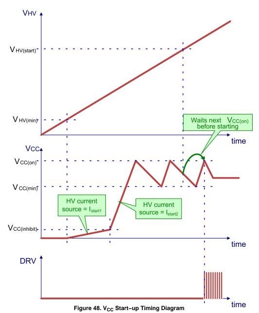
For safety reasons, the start–up current is lowered when  $V_{CC}$  is below  $V_{CC(inhibit)}$ , to reduce the power dissipation in case the  $V_{CC}$  pin is shorted to GND (in case of  $V_{CC}$  capacitor failure, or external pull–down on  $V_{CC}$  to disable the controller). There is only one condition for which the current source doesn't turn on when  $V_{CC}$  reaches  $V_{CC(inhibit)}$ : the voltage on HV pin is too low (below  $V_{HV(min)}$ ).
