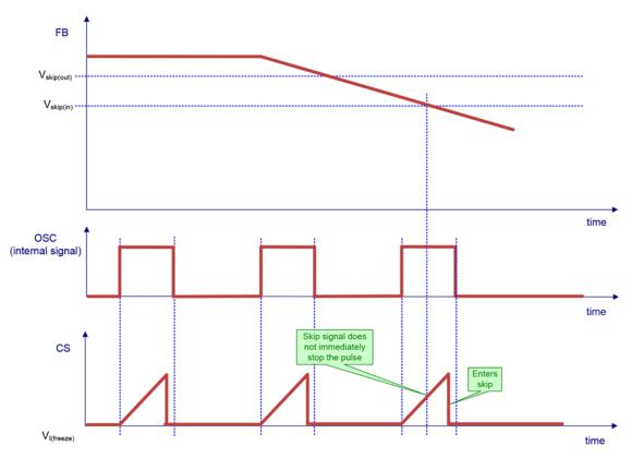
Figure 62. Technique Preventing Short Pulses in Skip Mode
