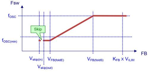
Figure 60. Frequency Foldback Mode Characteristic
