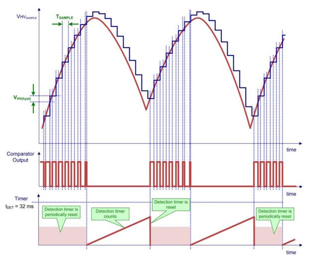
Figure 54. The ac Line Unplug Detector Timing Diagram
