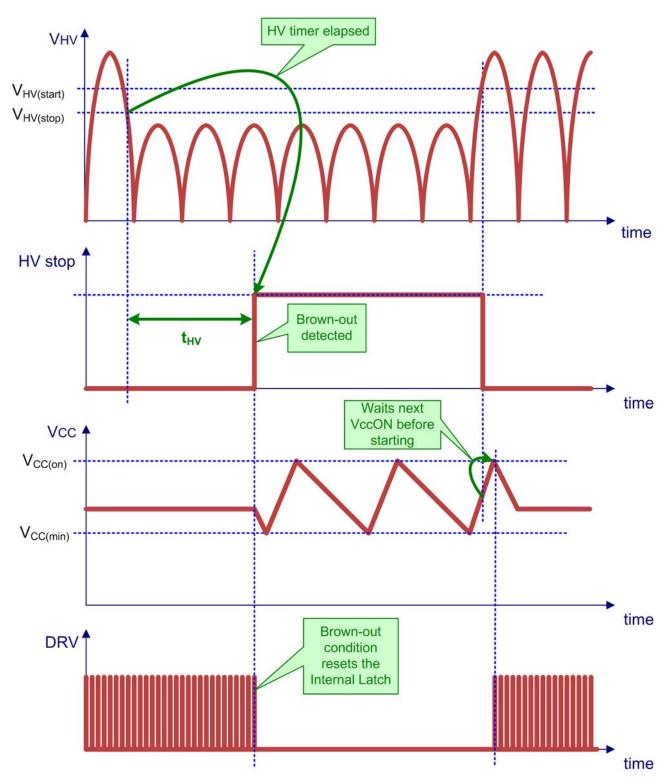
Figure 49. Ac Line Drop-out Timing Diagram
