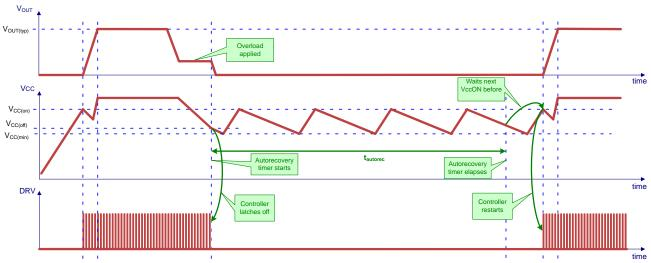
Figure 50.  $V_{\mbox{CC}}$  Collapses After Overload and Its Recovery
