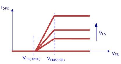
Figure 67. Overpower Protection Current Relation to Feedback Voltage
