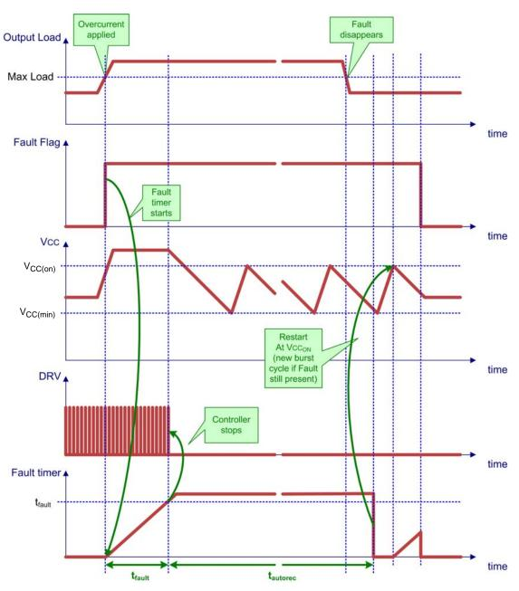
Figure 72. Timer-Based Protection Mode with Autorecovery Release from Latch-off (Options B/F)
