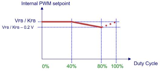
Figure 65. Slope Compensation Timing Diagram
