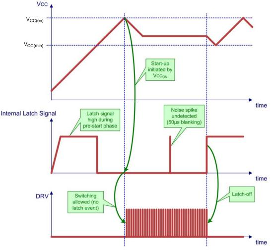
Figure 76. Latch Timing Diagram
