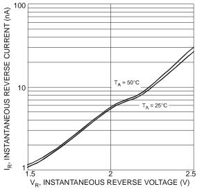
Figure 4 Typical Reverse Characteristics - GDZ5V1LP3
