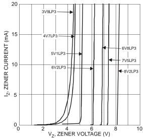
Figure 3 Typical Zener Breakdown Characteristics
