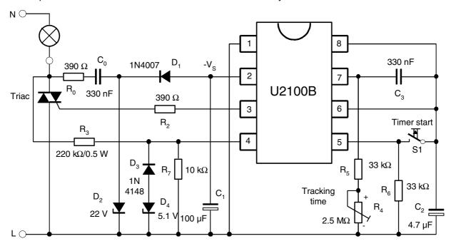
Figure 11. Fan Tracking Time Control 18 Seconds to 23 Minutes
