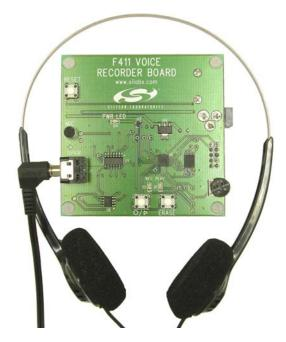
Figure 1. Voice Recorder Reference Design Board
