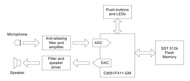
Figure 3. Voice Recorder Functional Block Diagram
