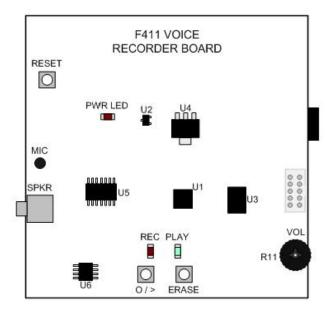
Figure 2. Voice Recorder Reference Design Components
