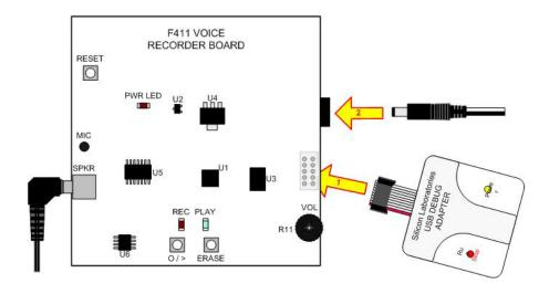
Figure 4. Voice Recorder Debugging Setup
