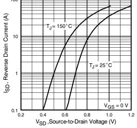
Fig 8. Typical Source-Drain Diode Forward Voltage
