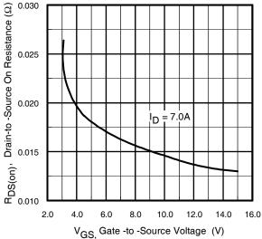
Fig 7. On-Resistance Vs. Gate Voltage
