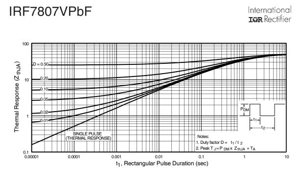
Figure 9. Maximum Effective Transient Thermal Impedance, Junction-to-Ambient
