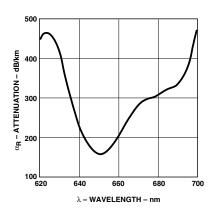
Figure 1. Typical POF attenuation vs. wavelength.
