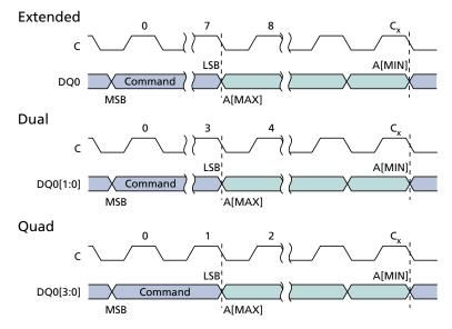
Note: 1. For extended SPI protocol,  $C_x = 7 + (A[MAX] + 1)$ . For dual SPI protocol,  $C_x = 3 + (A[MAX] + 1)/2$ . For quad SPI protocol,  $C_x = 1 + (A[MAX] + 1)/4$ .
