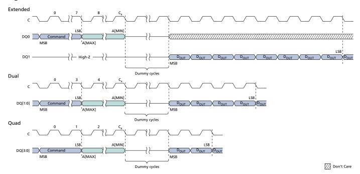
Note: 1. For extended protocol,  $C_x = 7 + (A[MAX] + 1)$ ; For dual protocol,  $C_x = 3 + (A[MAX] + 1)/2$ ; For quad protocol,  $C_x = 1 + (A[MAX] + 1)/4$ .
