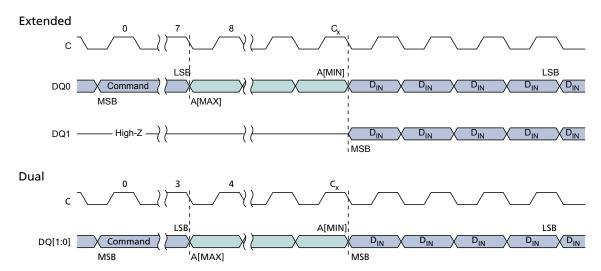
Note: 1. For extended SPI protocol,  $C_x = 7 + (A[MAX] + 1)$ . For dual SPI protocol,  $C_x = 3 + (A[MAX] + 1)/2$ .
