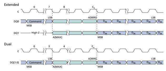
Note: 1. For extended SPI protocol,  $C_x = 7 + (A[MAX] + 1)/2$ . For dual SPI protocol,  $C_x = 3 + (A[MAX] + 1)/2$ .
