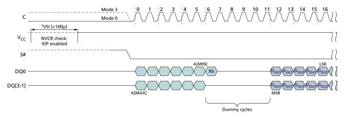
Note: 1. Xb is the XIP confirmation bit and should be set as follows: 0 to keep XIP state; 1 to exit XIP mode and return to standard read mode.
