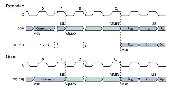
Note: 1. For extended SPI protocol,  $C_x = 7 + (A[MAX] + 1)/4$ . For quad SPI protocol,  $C_x = 1 + (A[MAX] + 1)/4$ .
