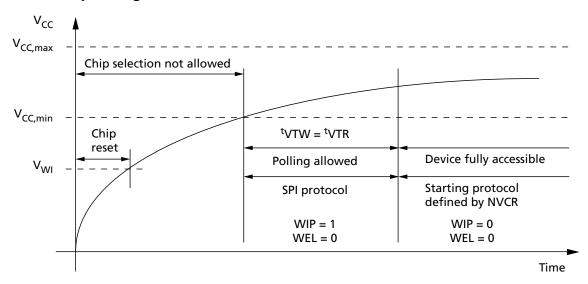
Table 30: Power-Up Timing and V<sub>WI</sub> Threshold
