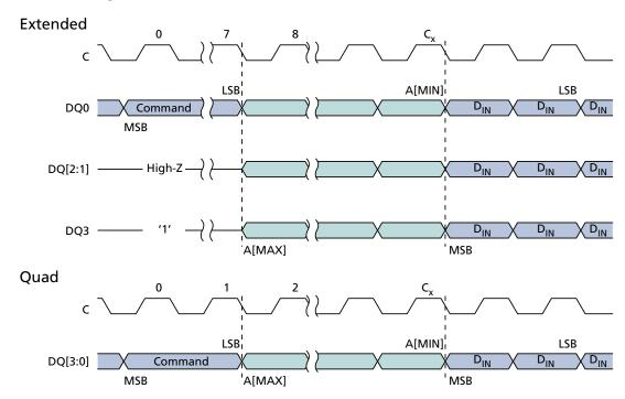
Note: 1. For extended SPI protocol,  $C_x = 7 + (A[MAX] + 1)/4$ . For quad SPI protocol,  $C_x = 1 + (A[MAX] + 1)/4$ .
