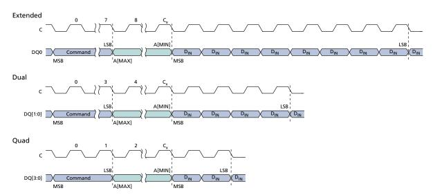
Note: 1. For extended SPI protocol,  $C_x = 7 + (A[MAX] + 1)$ . For dual SPI protocol,  $C_x = 3 + (A[MAX] + 1)/2$ . For quad SPI protocol,  $C_x = 1 + (A[MAX] + 1)/4$ .
