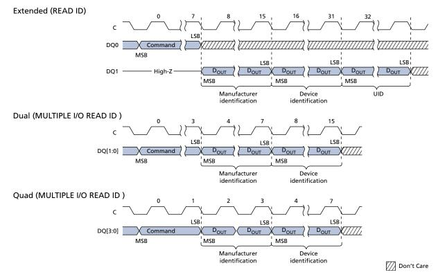
Note: 1. The READ ID command is represented by the extended SPI protocol timing shown first. The MULTIPLE I/O READ ID command is represented by the dual and quad SPI protocols are shown below extended SPI protocol.
