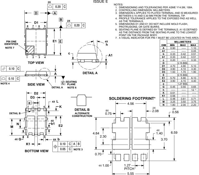
DIMENSION: MILLIMETERS \*For additional information on our Pb-Free strategy and soldering details, please download the ON Semiconductor Soldering and Mounting Techniques Reference Manual, SOLDERRM/D.
