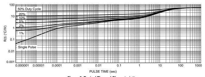
Figure 8. Typical Thermal Characteristics
