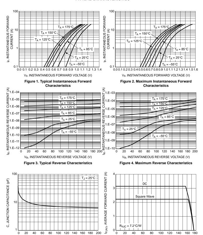
$\label{eq:VRRSEVOLTAGE} V_R\text{, REVERSE VOLTAGE (V)}$  Figure 5. Typical Junction Capacitance
