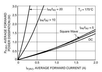
Figure 7. Forward Power Dissipation
