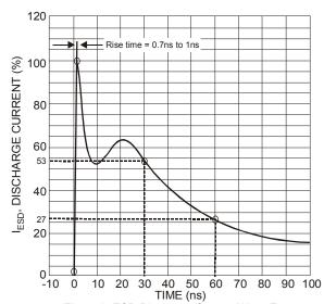
Figure 2 ESD Discharge Current Wave Form IEC 6100-4-2 (330\(\Omega\)/150pF)
