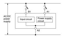
Since the input circuit and the power supply circuit are configured independently, the input circuit can be turned on or off irrespective of the on/off state of the power supply. Note that a voltage equivalent to the power supply voltage is applied to the input circuit.
