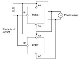
The H3DE Series is provided with a transformerless power supply system.
