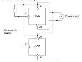
**Note:** The H3DE Series is provided with a transformerless power supply system.
