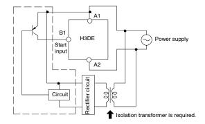
The H3DE-H has a large inrush current; provide sufficient power supply capacity. If the power supply capacity is too small, there may be delays in turning ON the output.
