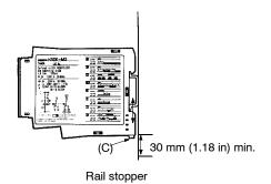
The H3DE can be mounted and removed easily if a distance of 30 mm (1.18 min) or more is kept between the H3DE and the top surface of other equipment located below the H3DE.
