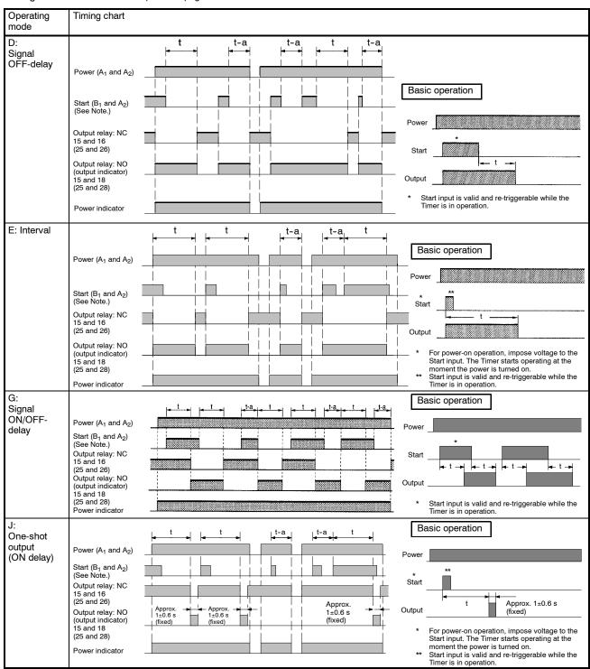
Note: The start input of the H3DE-M1 or H3DE-M2 model is activated by applying a voltage to B1 and A2 terminals.
