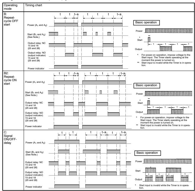
Note: The start input of the H3DE-M1 or H3DE-M2 model is activated by applying a voltage to B1 and A2 terminals.
