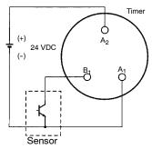
Operates with NPN transistor ON
