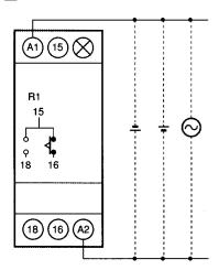
Note: DC supply voltage does not require the designation of polarity.
