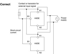
The H3DE Series is provided with a transformerless power supply system.
