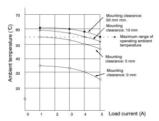
(Measurement Condition: Input voltage of 230 VAC)
