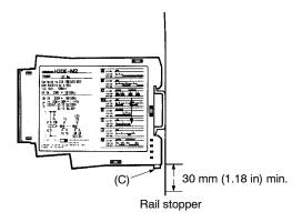
The H3DE can be mounted and removed with ease if a distance of 30 mm (1.18 in) or more is kept between the H3DE and the top surface of other equipment located below the H3DE.
