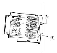
When removing the H3DE, pull out portion (C) with a flat-blade screwdriver and remove the Timer from the mounting track.
