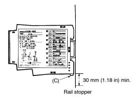
The H3DE can be mounted or removed easily if a distance of 30 mm (1.18 in) or more is kept between the H3DE and the top surface of other equipment located below the H3DE.
