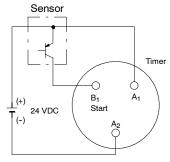
Operates with PNP transistor ON
