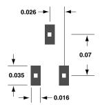
Figure 23. PCB Pad Layout, SOT-323. (dimensions in inches).
