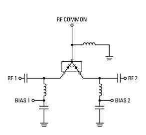
Figure 12. Simple SPDT Switch, Using Only Positive Current.
