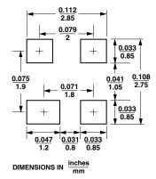
Figure 25. PCB Pad Layout, SOT-143.
