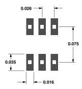
Figure 22. PCB Pad Layout, SOT-363. (dimensions in inches).
