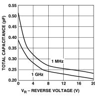
Figure 2. Capacitance vs. Reverse Voltage.
