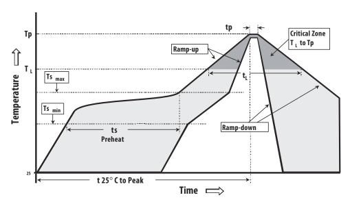
Figure 26. Surface Mount Assembly Profile.
