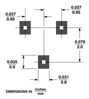
Figure 24. PCB Pad Layout, SOT-23.
