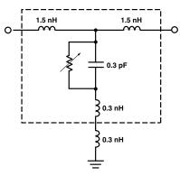
Figure 19. Equivalent Circuit.
