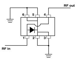
Figure 9. HSMP-389T used in a Low Inductance Shunt Mounted Switch.
