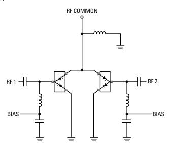
Figure 13. High Isolation SPDT Switch, Dual Bias.
