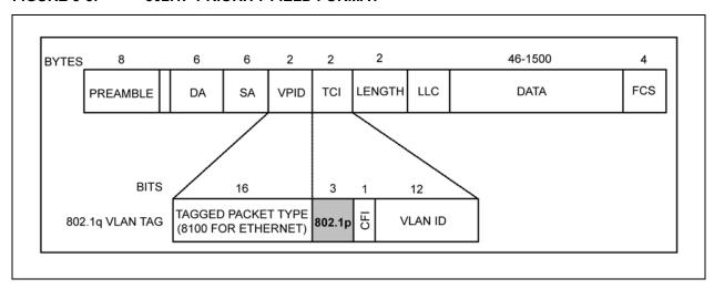
802.1p-based priority is enabled by bit [5] of the Registers Port Control 0 for ports 1, 2, 3, 4 and 5, respectively.
