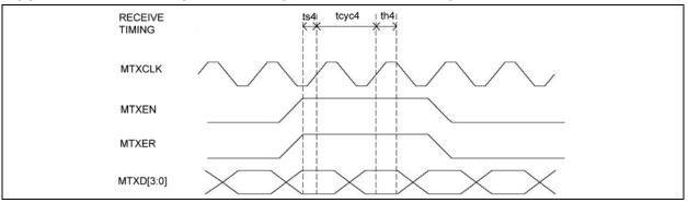
FIGURE 7-8: PHY MODE MII TIMING - DATA TRANSMITTED FROM MII
