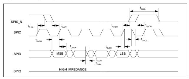
TABLE 7-6: SPI INPUT TIMING PARAMETERS
