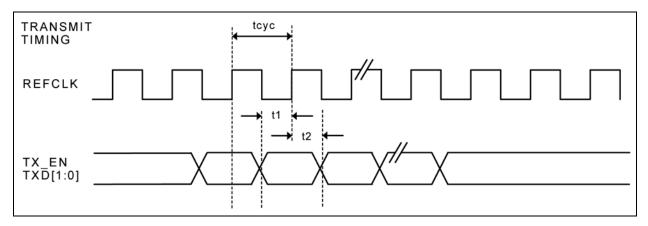
FIGURE 7-10: RMII TIMING - DATA TRANSMITTED TO RMII
