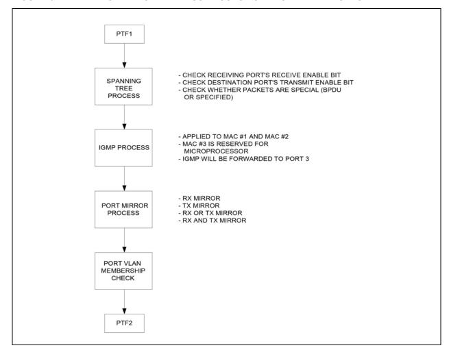
FIGURE 3-7: DESTINATION ADDRESS RESOLUTION FLOW CHART - STAGE 2
