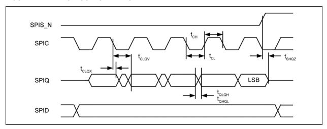
TABLE 7-7: SPI OUTPUT TIMING PARAMETERS
