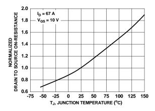
Figure 3. Normalized On-Resistance vs. Junction Temperature
