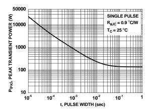
Figure 12. Single Pulse Maximum Power Dissipation
