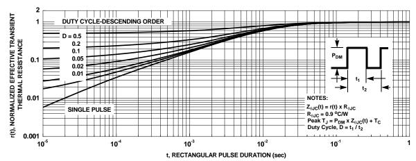
Figure 13. Junction-to-Case Transient Thermal Response Curve
