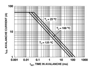
Figure 9. Unclamped Inductive Switching Capability
