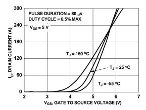
Figure 5. Transfer Characteristics
