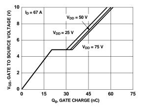
Figure 7. Gate Charge Characteristics
