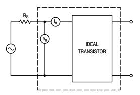
Figure 1. Transistor Noise Model
