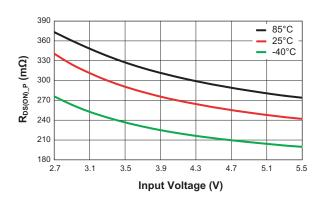
R<sub>DS(ON) N</sub> vs. Input Voltage
