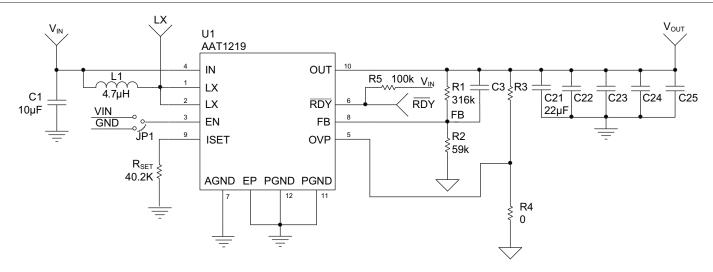
Figure 2: AAT1219 Evaluation Board Schematic.
