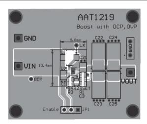
Figure 3: AAT1219 Evaluation Board Top Side Layout.
