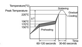
[Allowable Reflow Soldering Temperature and Time]
