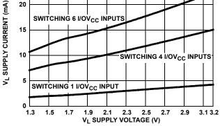
FIGURE 8. VL SUPPLY CURRENT vs VL SUPPLY VOLTAGE
