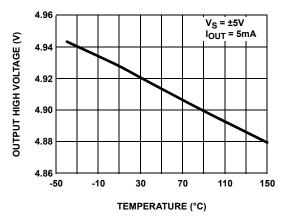
FIGURE 5. OUTPUT HIGH VOLTAGE vs TEMPERATURE
