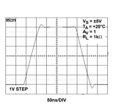
FIGURE 25. LARGE SIGNAL TRANSIENT RESPONSE
