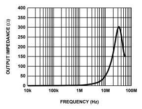
FIGURE 17. CLOSED LOOP OUTPUT IMPEDANCE
