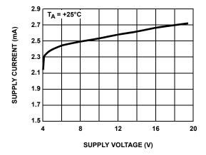
FIGURE 9. SUPPLY CURRENT PER AMPLIFIER vs SUPPLY VOLTAGE
