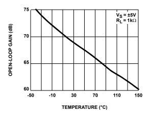
FIGURE 7. OPEN-LOOP GAIN vs TEMPERATURE
