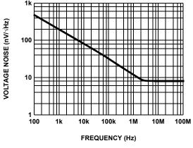
FIGURE 21. INPUT VOLTAGE NOISE SPECTRAL DENSITY
