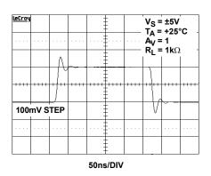
FIGURE 26. SMALL SIGNAL TRANSIENT RESPONSE
