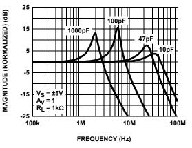
FIGURE 16. FREQUENCY RESPONSE FOR VARIOUS CL
