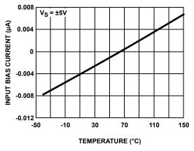
FIGURE 4. INPUT BIAS CURRENT vs TEMPERATURE
