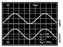
FIGURE 27. OPERATION WITH RAIL-TO-RAIL INPUT AND OUTPUT
