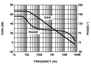
FIGURE 14. OPEN LOOP GAIN AND PHASE
