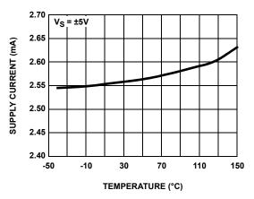
FIGURE 10. SUPPLY CURRENT PER AMPLIFIER vs TEMPERATURE
