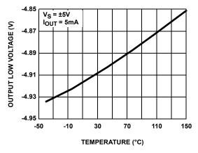
FIGURE 6. OUTPUT LOW VOLTAGE vs TEMPERATURE
