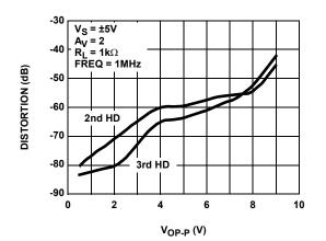
FIGURE 13. HARMONIC DISTORTION vs VOP-P
