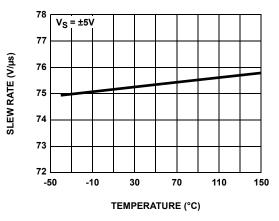
FIGURE 8. SLEW RATE vs TEMPERATURE
