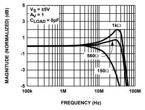
FIGURE 15. FREQUENCY RESPONSE FOR VARIOUS RL
