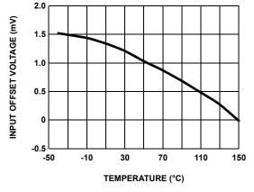
FIGURE 3. INPUT OFFSET VOLTAGE vs TEMPERATURE
