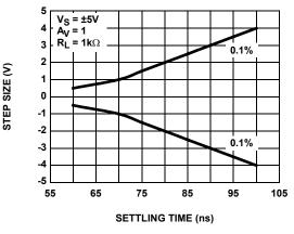
FIGURE 24. SETTLING TIME vs STEP SIZE
