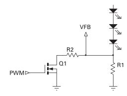
$$MOSFET 'off' \\ I_{LED(MIN)} = \frac{V_{FB}}{R_{LED}}$$
