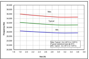
FIGURE 36-51: LFINTOSC Frequency, PIC16LF1615/9 Only.
