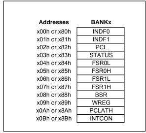
file registers) or indirectly via the two File Select Registers (FSR). See **Section 3.6 "Indirect Addressing**" for more information.
