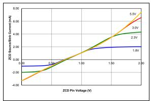
*FIGURE 36-109:* ZCD Pin Current over ZCD Pin Voltage, Typical Measured Values from -40°C to 125°C.
