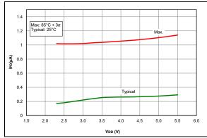
FIGURE 36-40: IPD, ADC Non-Converting, PIC16F1615/9 Only.
