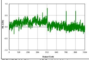
**FIGURE 36-74:** ADC 10-bit Mode, Single-Ended INL, VDD = 3.0V, TAD =  $4 \mu$ S,  $25^{\circ}$ C.
