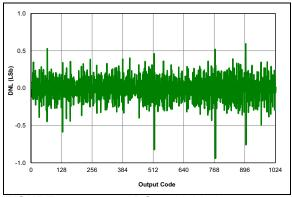
**FIGURE 36-72:** ADC 10-bit Mode, Single-Ended DNL, VDD = 3.0V, TAD =  $4 \mu$ S,  $25^{\circ}$ C.
