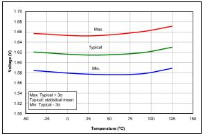
FIGURE 36-65: POR Release Voltage.
