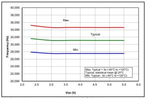
FIGURE 36-52: LFINTOSC Frequency, PIC16F1615/9 Only.
