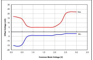
**FIGURE 36-90:** Comparator Offset, NP Mode (CxSP = 1), VDD = 3.0V, Typical Measured Values From -40°C to 125°C.
