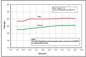
FIGURE 36-70: FVR Stabilization Period, PIC16LF1615/9 Only.
