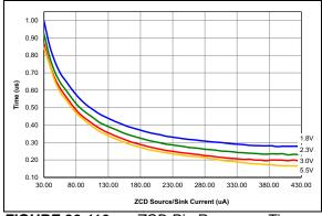
**FIGURE 36-110:** ZCD Pin Response Timer over Current, Typical Measured Values from -40°C to 125°C.
