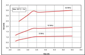
FIGURE 36-20: IDD Maximum, HFINTOSC Mode, PIC16F1615/9 Only.
