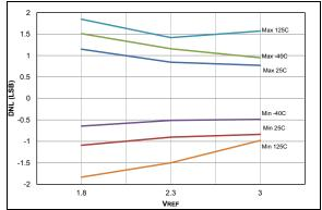
**FIGURE 36-77:** ADC 10-bit Mode, Single-Ended DNL, VDD = 3.0V,  $TAD = 1 \mu S$ .
