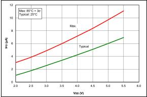
FIGURE 36-38: IPD, Timer1 Oscillator, Fosc = 32 kHz, PIC16F1615/9 Only.
