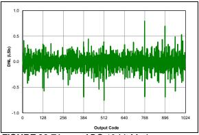
**FIGURE 36-71:** ADC 10-bit Mode, Single-Ended DNL, VDD = 3.0V,  $TAD = 1 \ \mu$ S, 25°C.
