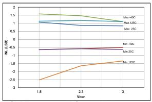
**FIGURE 36-78:** ADC 10-bit Mode, Single-Ended INL, VDD = 3.0V, TAD =  $1 \mu$ S.
