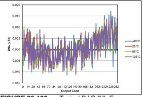
**FIGURE 36-100:** Typical DAC INL Error, VDD = 5.0V, VREF = External 5V, PIC16F1615/9 Only.
