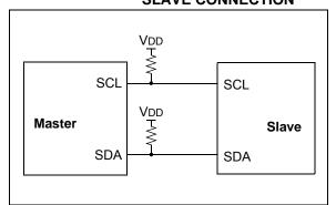
The Acknowledge bit  $(\overline{ACK})$  is an active-low signal, which holds the SDA line low to indicate to the transmitter that the slave device has received the transmitted data and is ready to receive more.
