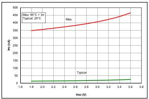
FIGURE 36-39: IPD, ADC Non-Converting, PIC16LF1615/9 Only.
