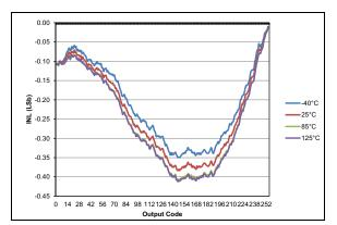
FIGURE 36-101: Typical DAC INL Error, VDD = 5.0V, VREF = External 5V, PIC16F1615/9 Only.
