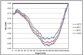
**FIGURE 36-99:** Typical DAC INL Error, VDD = 3.0V, VREF = External 3V.
