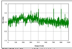
**FIGURE 36-73:** ADC 10-bit Mode, Single-Ended INL, VDD = 3.0V, TAD =  $1 \mu$ S,  $25^{\circ}$ C.
