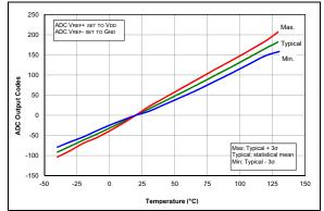
**FIGURE 36-87:** Temp. Indicator Slope Normalized to 20°C, High Range, VDD = 3.6V, PIC16LF1615/9 Only.
