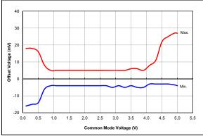
**FIGURE 36-93:** Comparator Offset, NP Mode (CxSP = 1), VDD = 5.5V, Typical Measured Values From -40°C to 125°C, PIC16F1615/9 Only.
