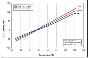
**FIGURE 36-86:** Temp. Indicator Slope Normalized to  $20^{\circ}$ C, Low Range, VDD = 3.0V, PIC16LF1615/9 Only.
