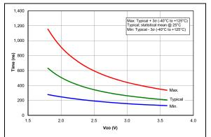
**FIGURE 36-96:** Comparator Output Filter Delay Time Over Temp., NP Mode (CxSP = 1), Typical Measured Values, PIC16LF1615/9 Only.
