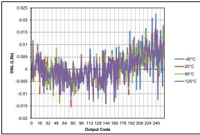
**FIGURE 36-98:** Typical DAC DNL Error, VDD = 3.0V, VREF = External 3V.
