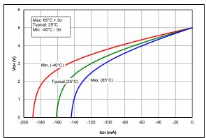
FIGURE 36-45: Voн vs. Ioн Over Temperature for High Drive Pins, Vdd = 5.0V, PIC16F1615/9 Only.
