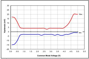
**FIGURE 36-92:** Comparator Offset, NP Mode (CxSP = 1), VDD = 5.0V, Typical Measured Values at 25°C, PIC16F1615/9 Only.
