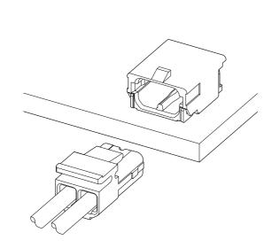
This SFK connector is a wire-to-board connector for connecting power supply and PCB and withstands high voltage. It is used for power supply of LED backlight in Liquid Crystal Display Television set.
