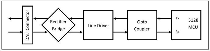
Figure 3: DALI interface circuit
