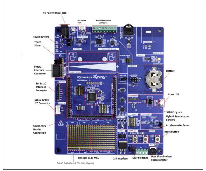
Figure 1 Main board components, top side
