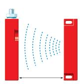
Encapsulated in the MA Series is a unique high-power industrial reed which is de-rated by a non-resetable overload protection circuit depending on switch type. On presenting the actuator to the switch, the high intensity magnetic field from the actuator causes the contacts to close. On removing the actuator (opening the door), the safety contacts open, isolating the machine.
